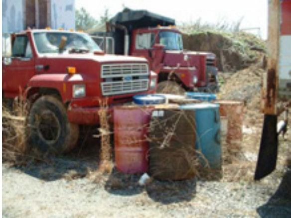
HS-1-2A and HS-2-2 At Park East Ventures (left) no pollutant source was confirmed, but rusty, uncovered fuel storage tanks and oil/antifreeze barrels were placed near a highly eroding area. At B & R Construction (right), unlabelled barrels contained unknown materials.
